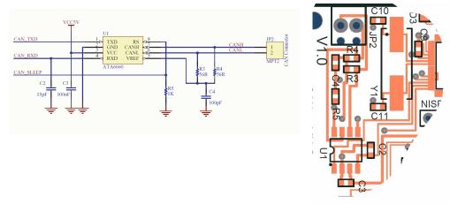
Figure 2-5. CAN High Speed connections
